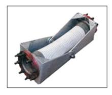
The flexible hose is a composite hose assembly with ASA # 150 flanges. The composite hose is designed with inner and out stainless steel helix that supported the internal multiple layers of elastomeric material. The inner and outer wire support make the hose non collapsible. The flanges are swaged over a Nipple and Ferrule. Hence there is no welding on the hose assembly. This hose assembly does not allow any permeation and is 100% aromatic resistant.
